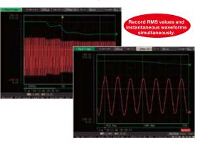
Maximum recording time is inversely proportional to number of recording analog channels.
