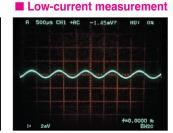
Input: 1 kHz sine wave 10 mAp-p (Oscilloscope bandwidth 20 MHz)
