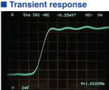
Input: 100 mAp-p (Oscilloscope bandwidth 400 MHz)
