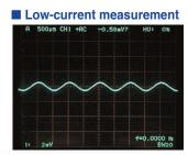
Input: 1 kHz sine wave 10 mAp-p (Oscilloscope bandwidth 20 MHz)
