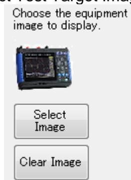
Click the [Select Test Target Image] button to select the desired image for the test target. In addition to being shown in the test target image area, the selected image will be output on PDF reports.
