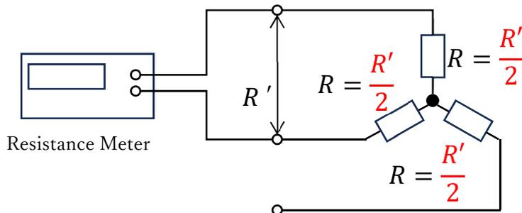
Connect the resistance meter to the motor as shown in the diagram and measure the DC resistance  $R'$  [ $\Omega$ ]. Calculate the phase armature resistance R using the following formula.
