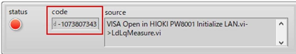
Please check if the IP address is correct, if the LAN is properly connected, and if NI-VISA is installed.
